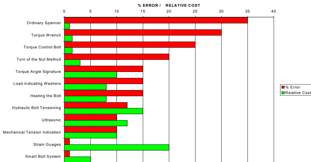
Figure 12: Comparison of common tightening methods
